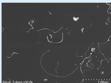
TiNa was developed especially for the application of nanomaterial detection, which requires SEM images with a field of view of 42.2  $\mu\text{m}$  x 31.7  $\mu\text{m}$  with a pixel size of 8.2 nm at random sample positions. The aim is to do an automated statistical based detection and classification of nanomaterials as harmful to health.
