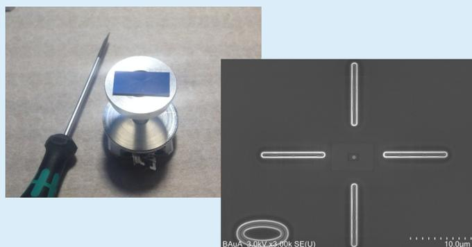
Fig. 2: left silicon test chip in the sample holder, right one control mark
